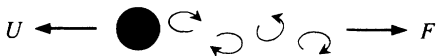
FIG. 2. A sphere moving at speed U through a viscous fluid must have a force acting on it to maintain its motion. The energy dissipation rate in the fluid is, on average, the product of the average force times the speed FU .
